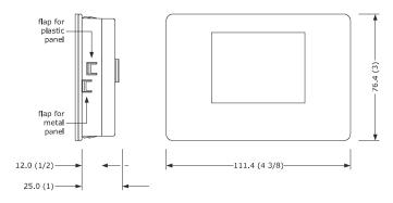
To be fitted to a panel, with elastic holding flaps.
