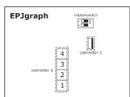
N. DESCRIPTION 1 CAN port reference -CAN port reference + device power supply (24 VAC/12... 30 VDC). If the device is fed by DC power, connect terminal minus
